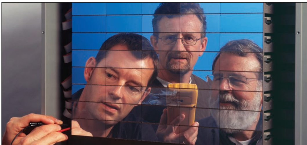
Fig. 3. The PILATUS 6M detector is a highly sensitive digital X-ray camera that consists of 60 modules with 6 million pixels, making up an active area of 43 cm x 45 cm. A spin-off company has been created to meet the growing demands in the field of synchrotron radiation. Members of the team are reflected here. Left to right: Christian Broennimann, Markus Naef and Eric Eikenberry.
