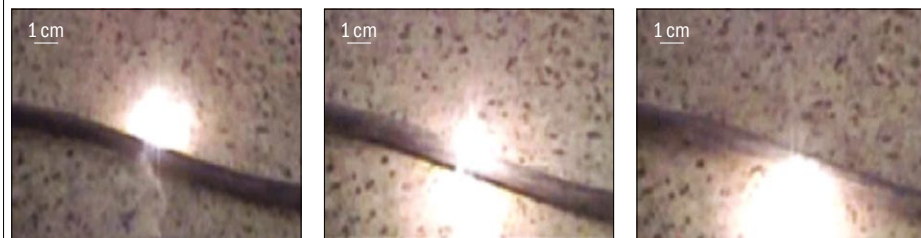
Successive video frames in which a luminous ball squeezes under an electrical conductor.
