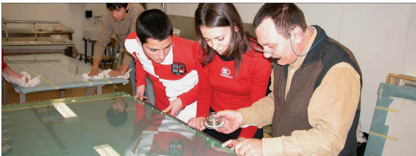
High-school students at CERN prepare the multigap resistive plate chambers, which are used in schools in the EEE Project.
