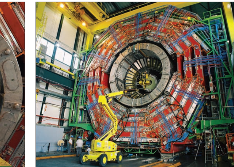
Left: a “gold plated” event, reconstructed online, from the CMS cosmic challenge. Right: preparing for the cosmic challenge. Muon chambers fill the detector. Two sectors of these chambers were fully equipped and used for the cosmic challenge. The ECAL supermodules used are visible behind the person working on the HCAL; gold coloured) and the solenoid cryostat (silver ring).
