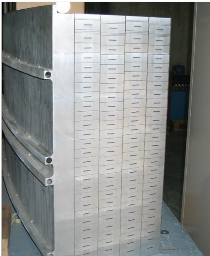
Fig. 2 (above) A model of the CMS solenoid coil, showing its four-layer coil-winding structure. Fig. 3 (above right). The solenoid, right, about to be inserted into the cryostat barrel. Fig. 4 (right). The first cool-down of the solenoid during three weeks in February 2006 was a complete success.
